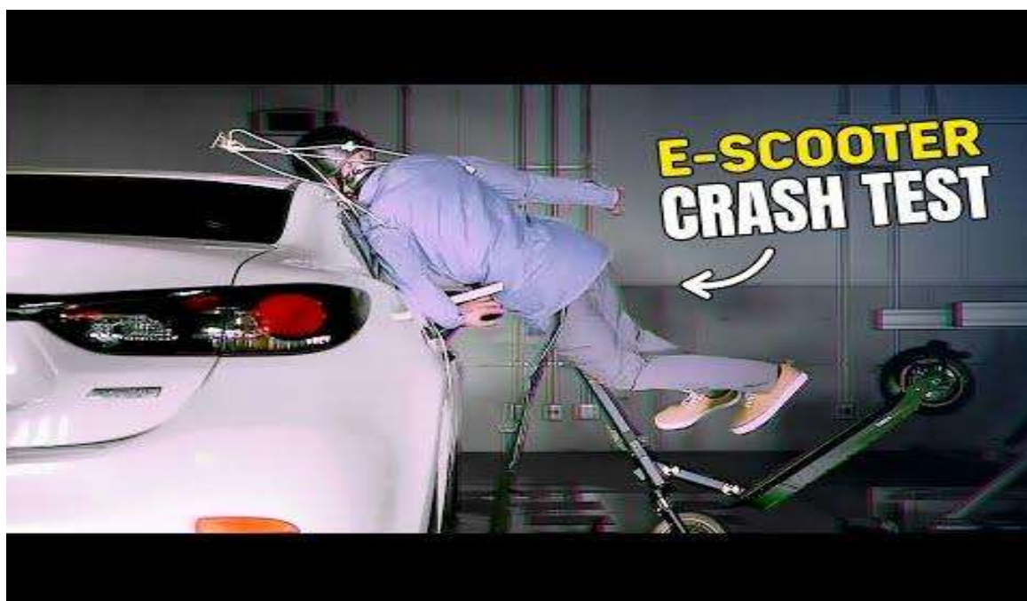
Figure 4: Japanese Automobile Federation – stand up e-scooter crash test dummy
